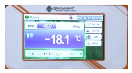
This is a temperature control unit designed for precise cooling applications. The touchscreen interface displays real-time temperature monitoring and settings. The different parameters display different functions in the control panel.
